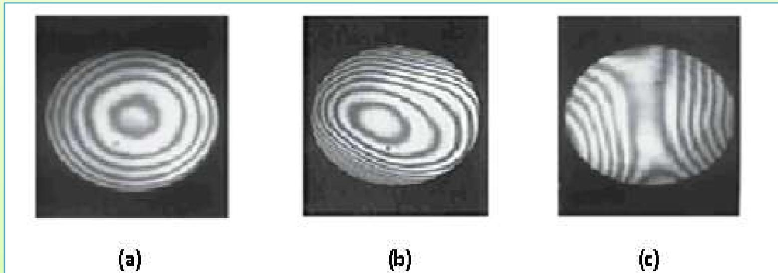
**Figure16: Testing the lens surface using Newton's rings (a) circular ring pattern indicating the perfectness of the surface (b) and (c) distorted patterns indicating irregularities**
