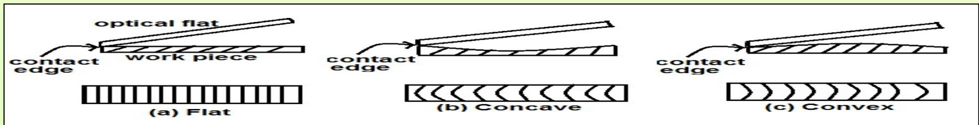
Figure10: Testing of surface finish (a) optically flat (b) concave (c) convex surface
