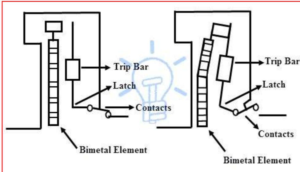
Under overload condition, the current through the bimetal causes to raise the temperature of it. The heat generated within the bimetal itself enough to cause deflection due to thermal expansion of metals. This deflection further releases the trip latch and hence contacts get separated. In some MCBs, magnetic field generated by the coil causes develop pull on bimetal such that it deflection activates the tripping mechanism.
