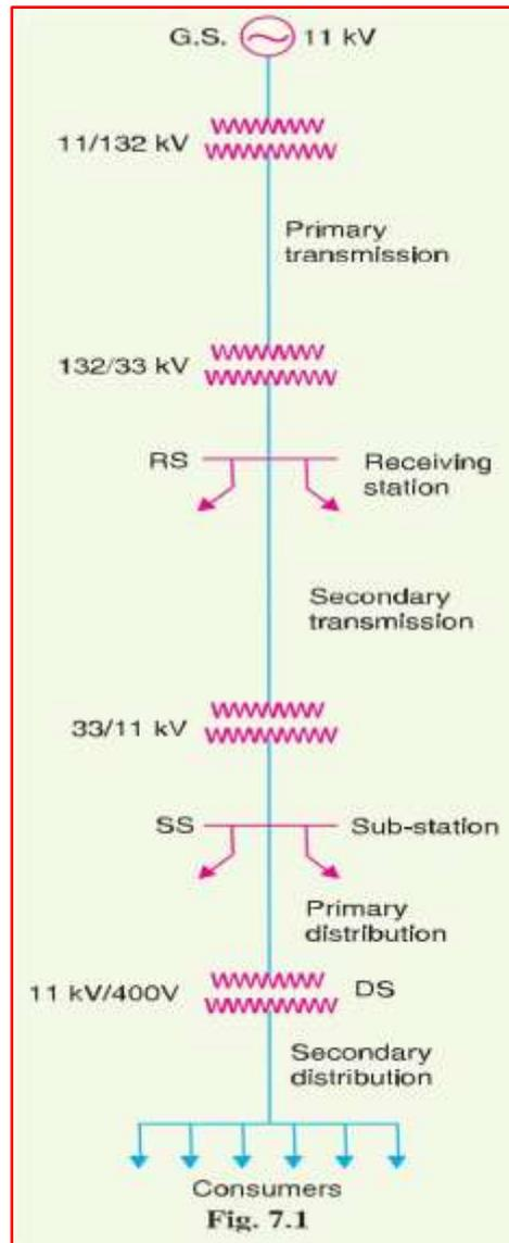
(i) **Generating station (G.S.):**- here electric power is produced by 3-phase alternators operating in parallel. The usual generation voltage is 11 kV. For economy in the transmission of electric power, the generation voltage (i.e., 11 kV) is **stepped upto 132 kV** (or more) at the generating station with the help of 3-phase trans-formers.
