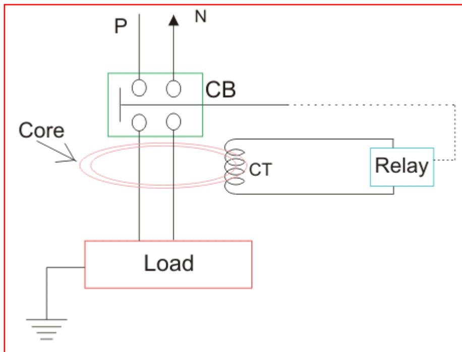
Single Phase Residual Current ELCB. The polarity of the phase winding and neutral winding on the core is so chosen that, in normal condition mmf of one winding opposes that of another. As it is assumed that, in normal operating conditions the current goes through the phase wire will be returned via neutral wire if there's no leakage in between. As both currents are same, the resultant mmf produced by these two currents is also zero-ideally.
