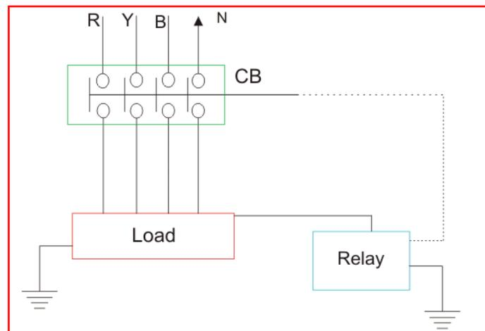
If the voltage difference crosses, a predetermined limit, the current through the relay becomes sufficient to actuate the relay for tripping the associated circuit breaker to disconnect the power supply to the equipment. The typicality of this device is, it can detect and protect only that
