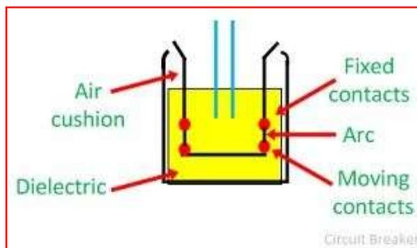
Whenever a fault occurs on any part of the system, the trip coil of the breaker gets energized and the moving contacts are getting apart from each other by some mechanism, thus opening the circuit.
