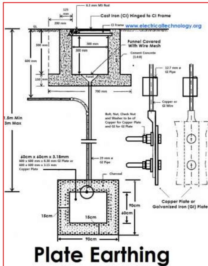
thickness of about 15cm. The earth wire (copper wire for copper plate earthing and G.I. wire for G.I. plate earthing) is securely bolted to an earth plate with the help of bolt, nut, and washer made of copper, in case of copper plate earthing and of G.I. in case of G.I. plate earthing.
